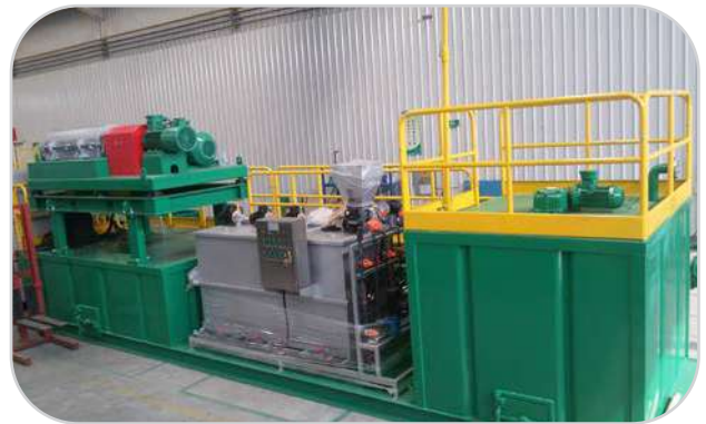
Cnooc 5 m 3 Slurry Treating System
