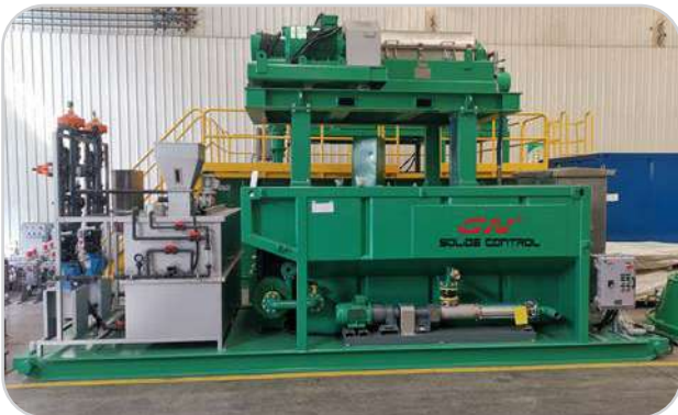
Sinopec 5 m 3 Slurry Treating System
