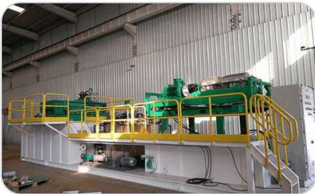
Shanghai 5 m 3 Slurry Treating System
